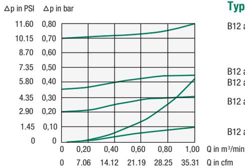
**Type SPB-3 (into / out of the tank)**
