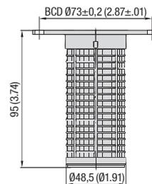
Six-hole bolt pattern with flange interface according to DIN 24557, part 2
