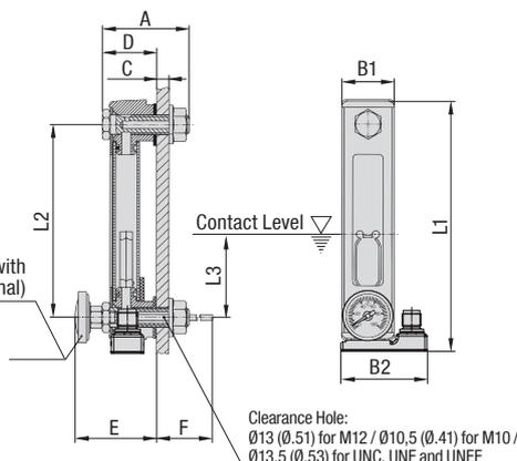
Clearance Hole:  $\varnothing 13$  ( $\varnothing 0.51$ ) for M12 /  $\varnothing 10.5$  ( $\varnothing 0.41$ ) for M10 /  $\varnothing 13.5$  ( $\varnothing 0.53$ ) for UNC, UNF and UNEF
