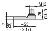
1 Contact opens and 1 contact closes when fluid level drops below contact level
