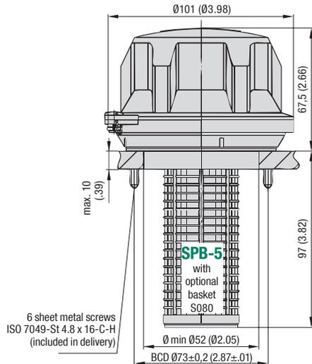
Installation to a six-hole bolt pattern
